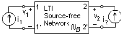
Fig. 16.1-6 Circuit in Fig. 16.1-3 reduced to a linear two-port driven by two current sources
